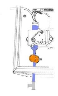
The 1/4" Barbed Equal T Fitting is attached to the drain.
