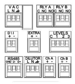
To connect ED4 to the TOC Analyzer, turn off the analyzer and open the right compartment. Remove the protective covering to access the user contacts. Insert all cables through the glands on top of the analyzer.
