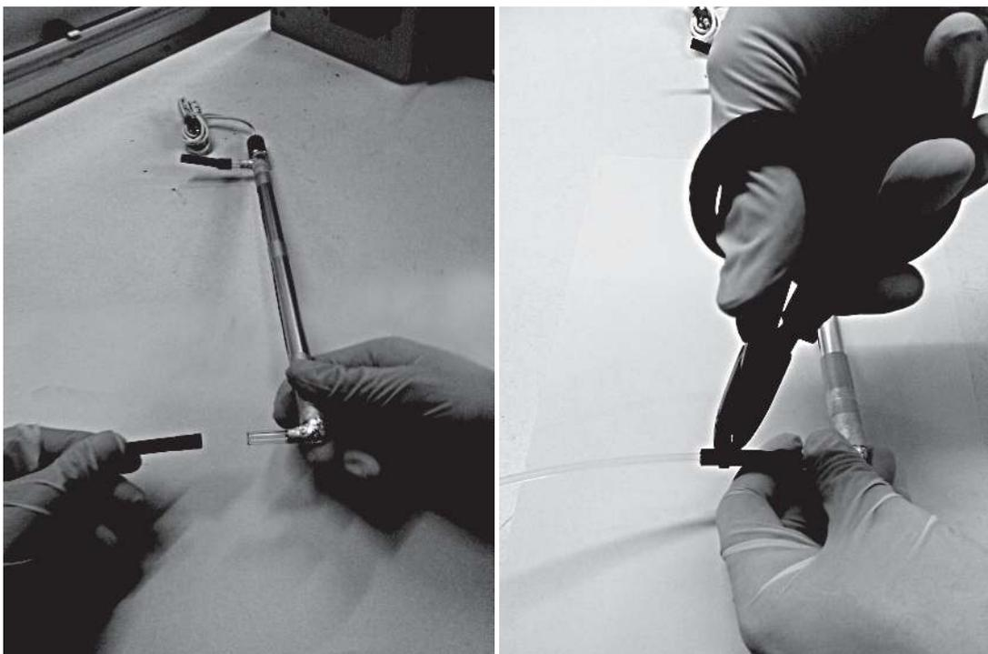
E - The Teflon tubing should be inserted inside the quartz inlets/outlets of the UV lamps, taking care not to impede the liquid flow.
