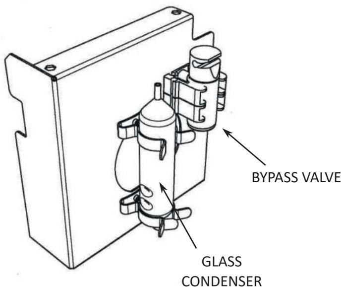
The bypass valve blocks the gas stream avoiding it to flow through the IR cell when not strictly necessary.
