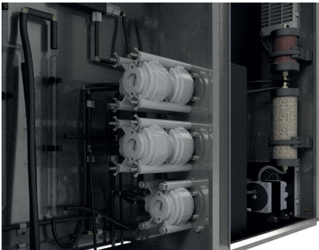
D - Disconnect each pump tubing from their inlet and outlet fittings, taking care to note which fitting will be needed to reconnect to which pump.
