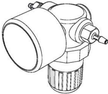
These devices are located in the central part of the electrical enclosure with a pressure gauge on the front and are used to supply a precise and reliable adjustment for the carrier gas flow.
