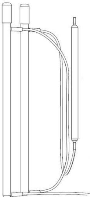
The UV reactor consists of two high energy UV lamps. The reaction of oxidation is catalyzed by UV radiation with decomposition of sodium persulfate and creation of strongly oxidizing radicals. These conditions ensure the best recovery of organic substances present in the sample. The second UV lamp is connected to UV scrubber. The oxidized sample at the UV lamps is sparged inside this device.
