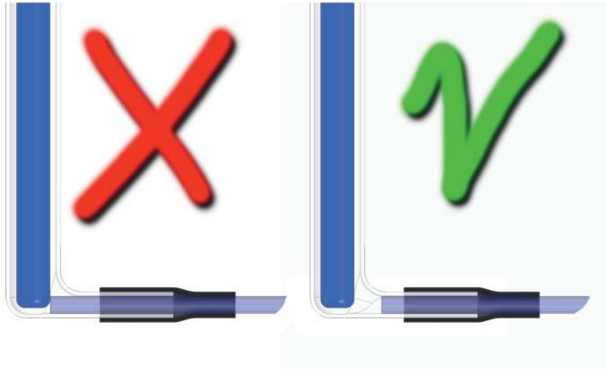
F - The norprene tubing should cover the Teflon tubing and the arm of the quartz inlets/outlets of the UV lamp
