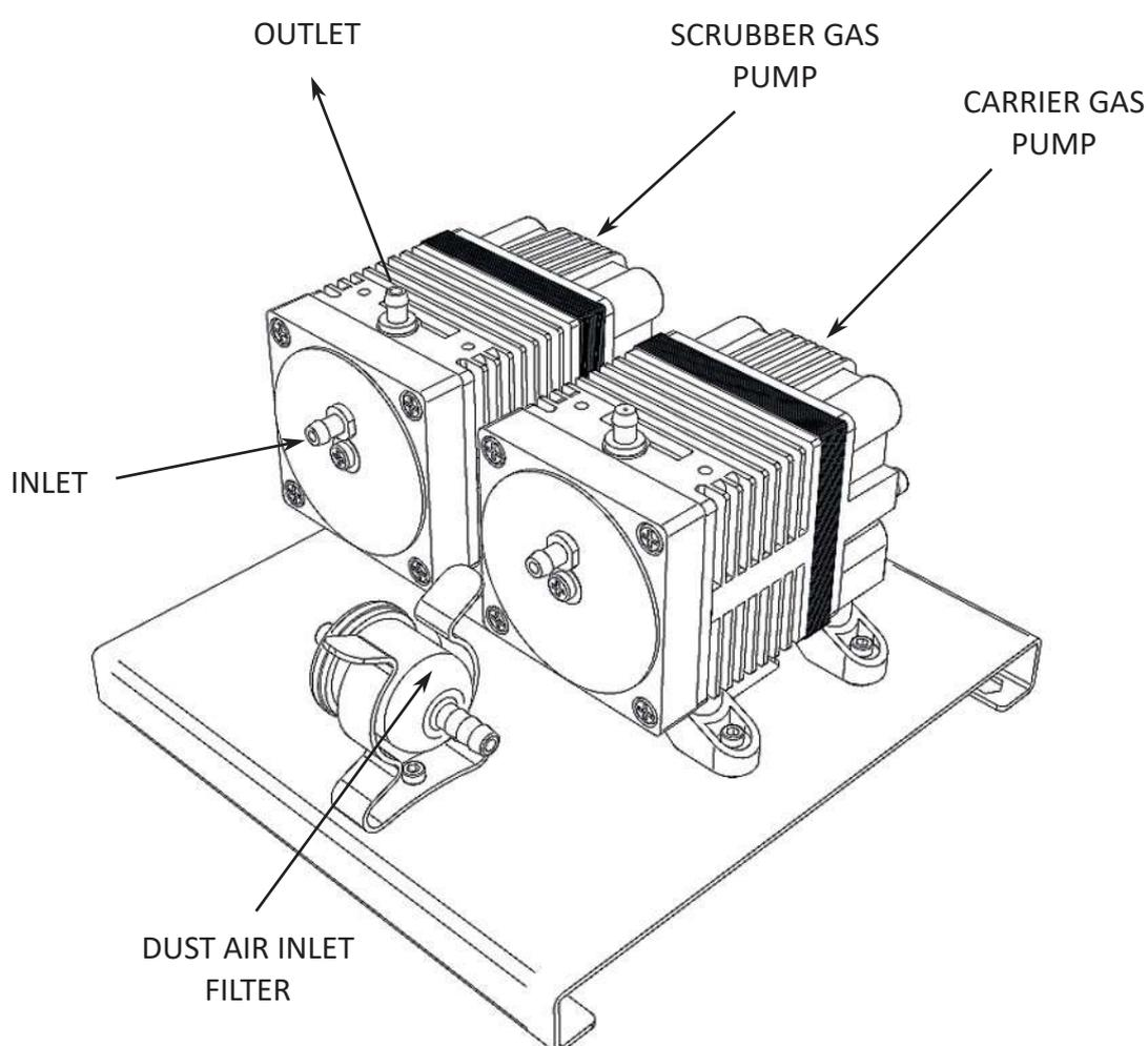
As pumps accessories there is a dust inlet paper filter and an electrical fan blows on the air pumps surface to cool them.
