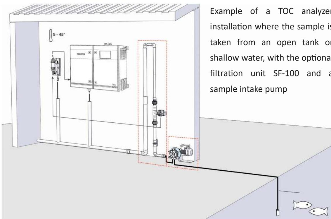
Example of a TOC analyzer installation where the sample is taken from an open tank or shallow water, with the optional filtration unit SF-100 and a sample intake pump
