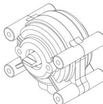
The **phosphoric acid pump** head is driven by the M2 (see section 3.11) motor and is located in the middle position, closest to the motor. It pumps phosphoric acid from the phosphoric acid container to the T fitting connected to sample pump head.
