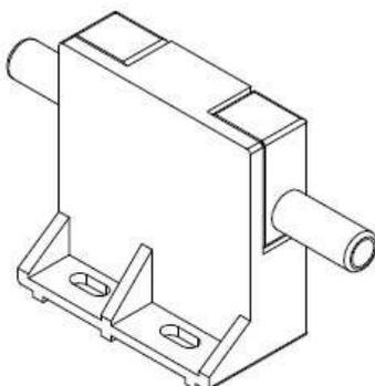
A mass thermal flowmeter provide the value of the carrier gas flow.
