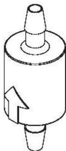
To prevent liquid back flow from the Liquid left compartment, a couple of Check valves are mounted on the two gas lines.
