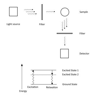
A polychromatic light source is filtered to select a specific wavelenght. Molecules in the sample absorb the energy from the radiation and reach Excited State 1.
