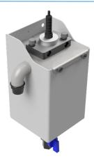
The 3S-TRB turbidity probe shown above is installed in the Fast Loop sample reservoir, protected from external light and easily accessible for cleaning and maintenance (the reservoir is compatible with all 3S probes, has to be purchased separately, product code A46U10035).
