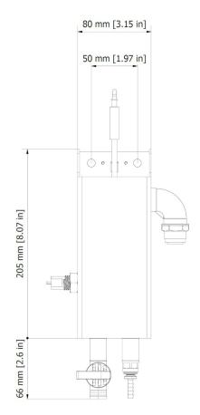
The reservoir can be mounted on the wall next to the analyzer, preferably on the right side of 3S-CL and 3S-UV models and on the left side of 3S-TM models.
