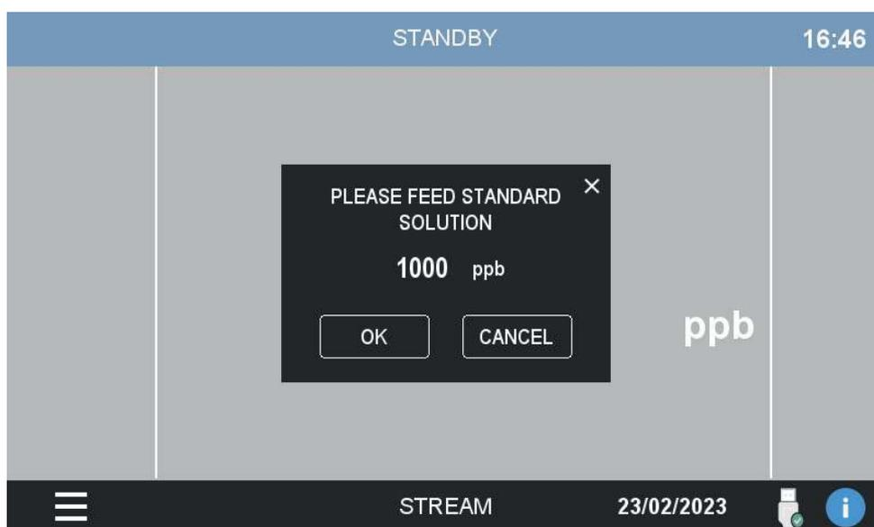
At the end of the countdown the calibration is completed. The outcome of the calibration can be checked in the DATALOGGER > CAL LOG.
