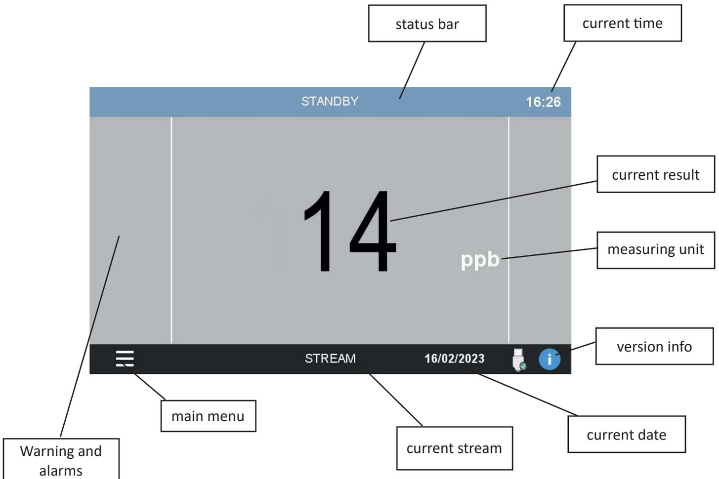
If the device was set to analyze 2 channels, you'll see an additional result value for channel B.
