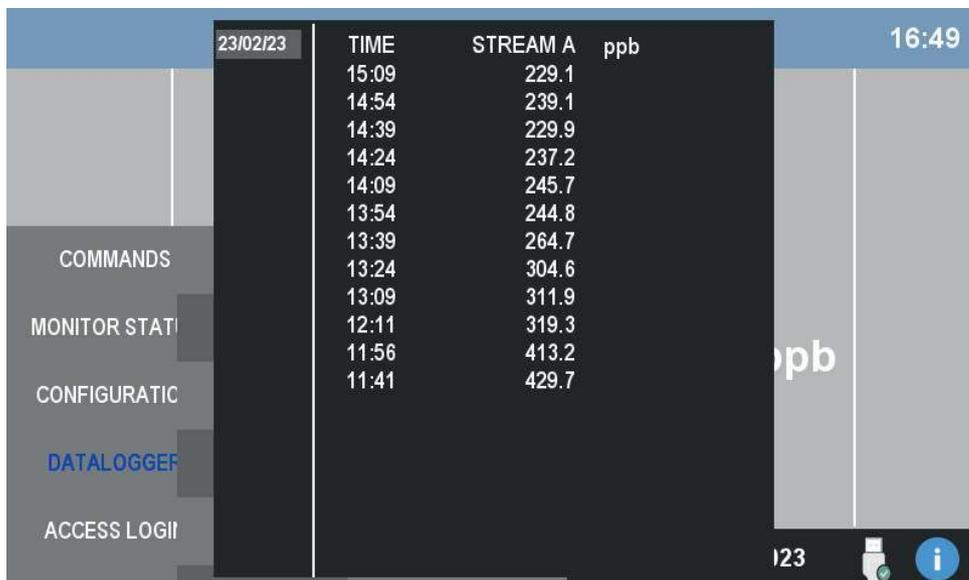
In the leftmost column there are the dates the data has been recorded on. By selecting a day the corresponding lists of measures will be displayed. The time column indicates the analysis time while the other two columns contains the data for the channel.
