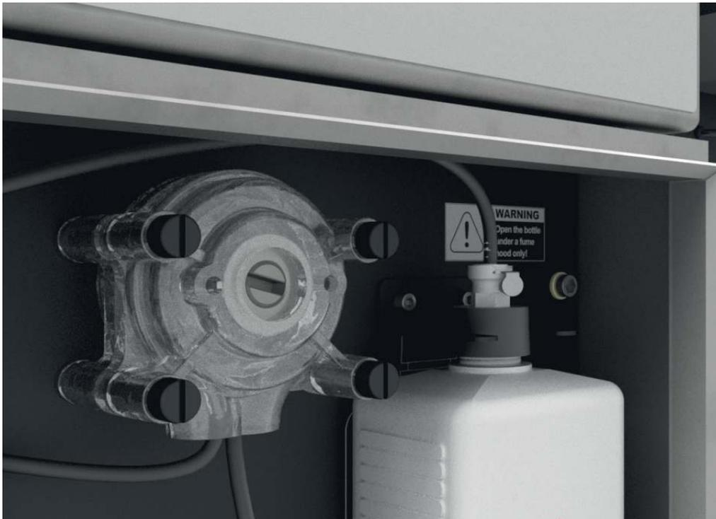
The reagent is required to adjust the pH. At low pH the hydrogen ion interferes with the electrode and gives false responses.
