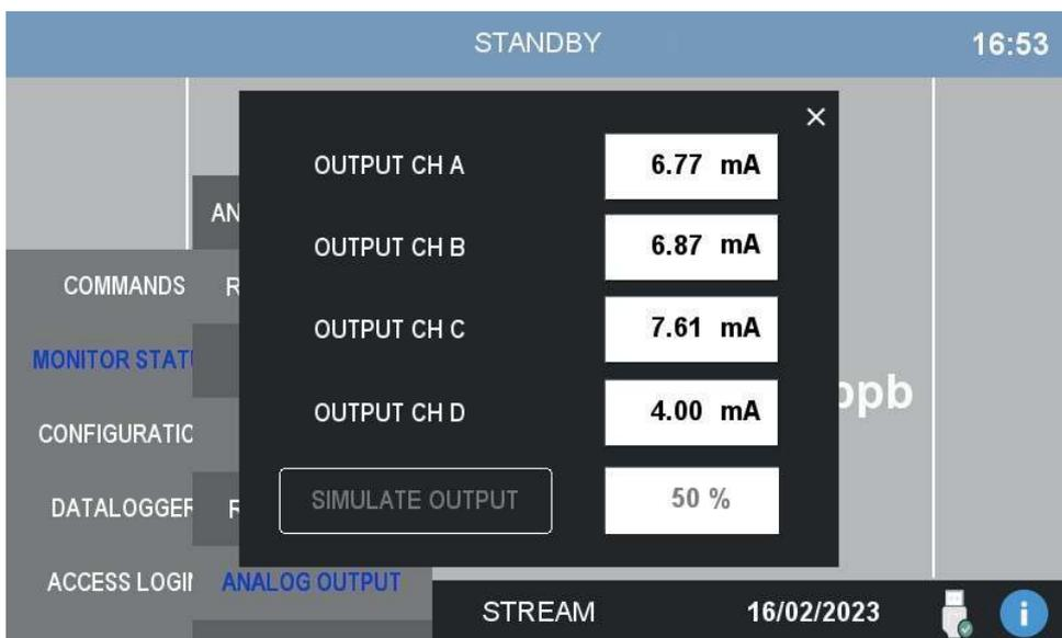
From the same window is also possible to simulate the output, this is useful to test a new installation or for servicing purposes.
