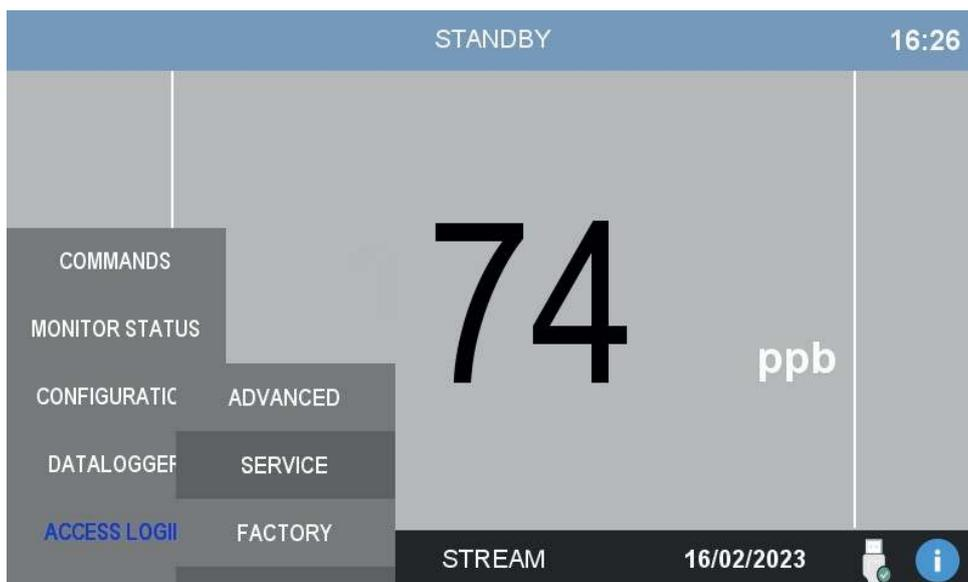
The analyzer has three levels of security, each level allows the user to access more advanced functions. The three levels are:
