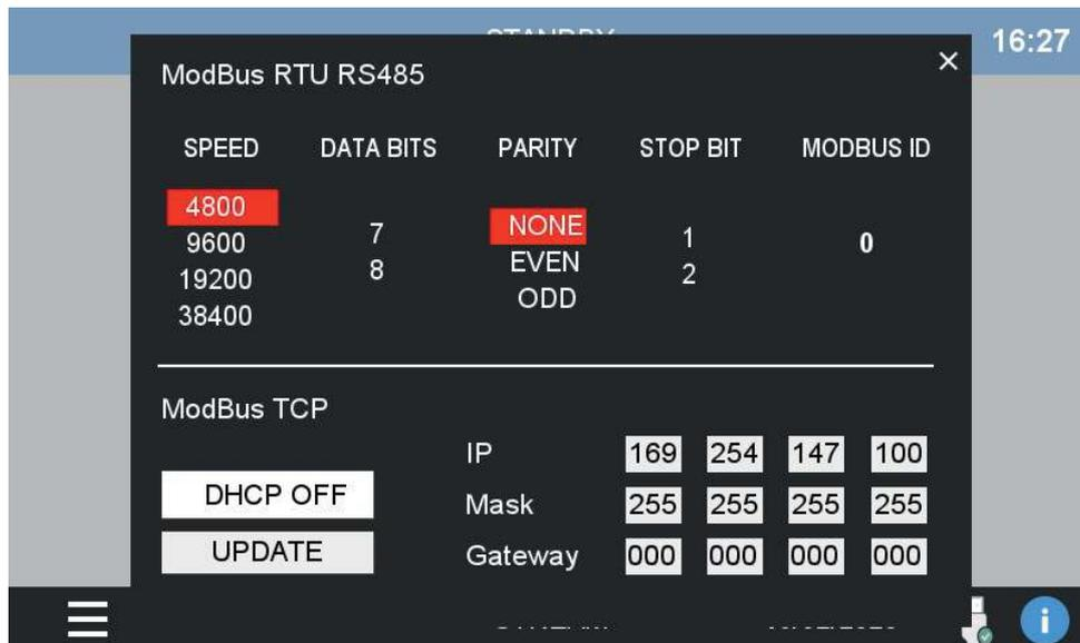
From here you can change the configuration parameter for the Modbus connection. In the upper part you can find the configuration of the connection via RS485, in the bottom part you can set the Ethernet parameters. You are free to set a static IP address or let DHCP decide, in any case remember to press UPDATE after any changes are made.
