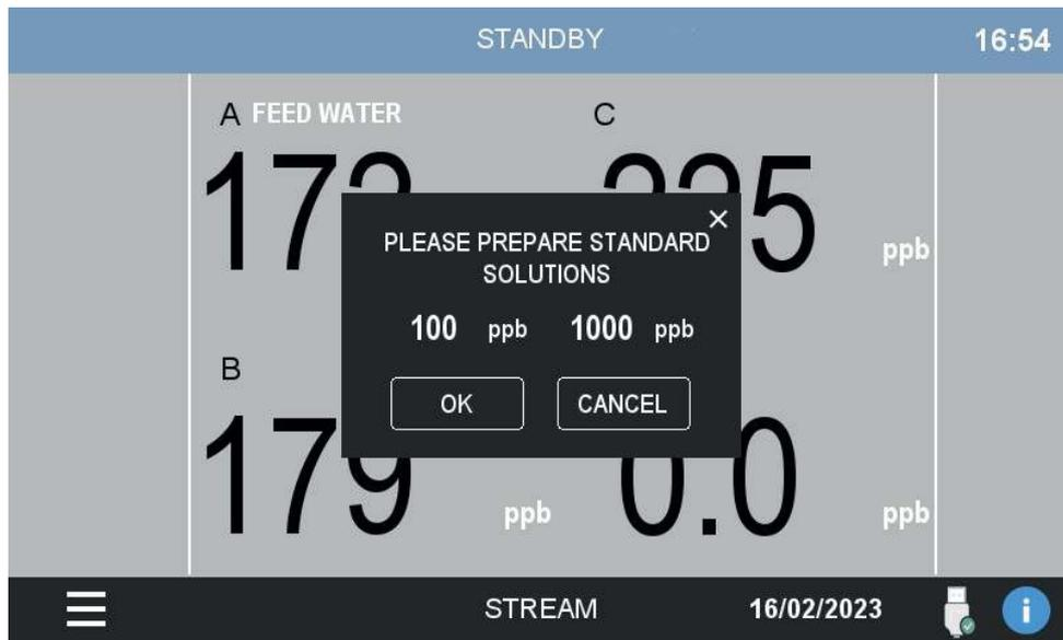
After confirmation, the calibration starts and the following window will be shown for the duration of the operation. If the window is closed before the calibration ends, the operation will be aborted.
