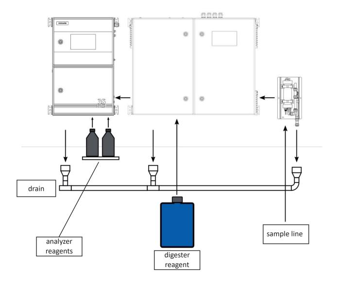
The installer should also provide a drain line without any backpressure to allow the free flow of liquids.
