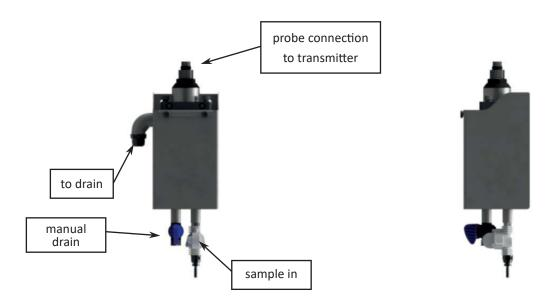
The sample reservoir can be mounted preferably under the instrument. The sample line must be connected to the inlet below the container, optionally a flow sensor can be installed on the same line to detect the presence of the sample.
