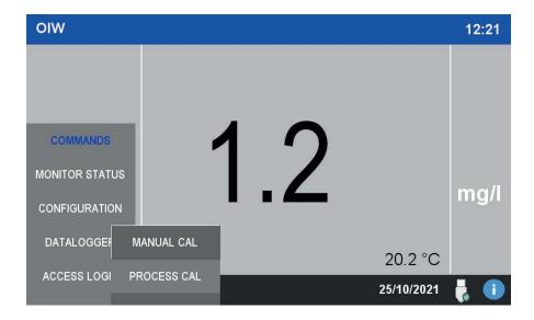
The COMMANDS menu contains the two commands to perform the calibrations. Both MANUAL CAL and PROCESS CAL will be discussed in details in the next chapter.
