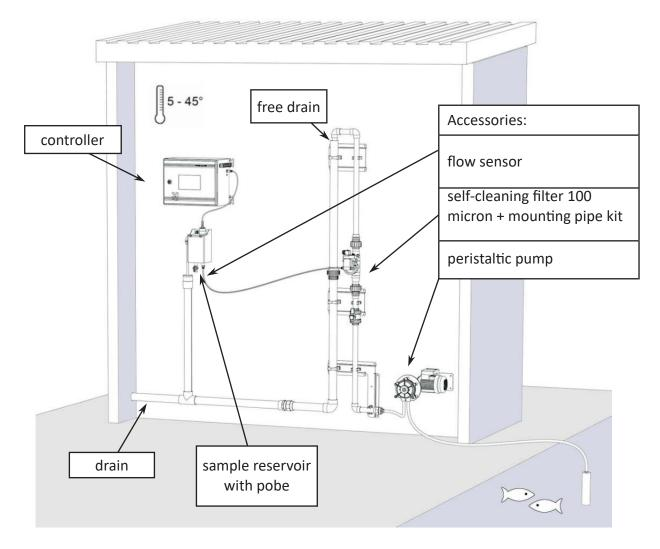
In the example, a large sample quantity is sucked by a peristaltic pump from an underlying head and sent to a self-cleaning filter.
