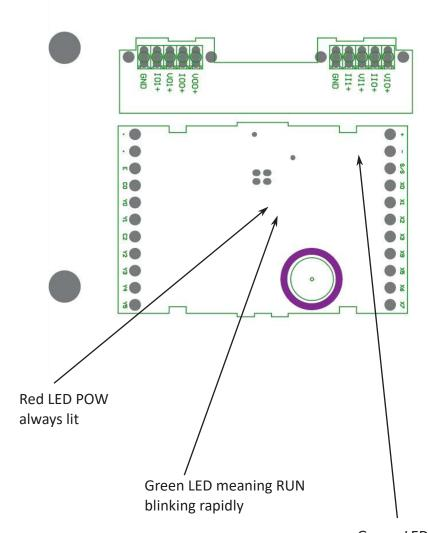
Green LED and red LED alternate and fast blinking showing the serial communication with the touchscreen panel
