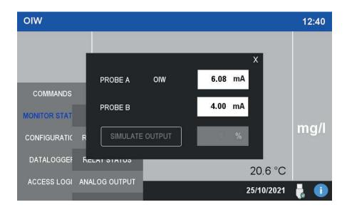
From this window the user can also simulate the analog output by inserting an arbitrary value in the SIMULATE OUTPUT field. This is useful for troubleshooting or mantainace purpose.
