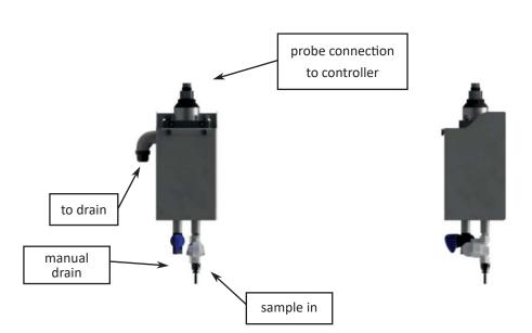
The sample reservoir (cod. A46U10035) should be mounted preferably under the controller. The sample line must be connected to the inlet below the container, optionally a flow sensor can be installed on the same line to detect the presence of the sample.
